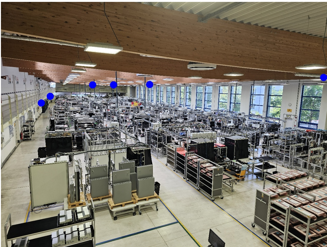
Figure 11: Locations of pRRHs inside of the production hall (blue dots).
